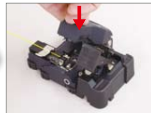
Push top cover to cleave the fiber
